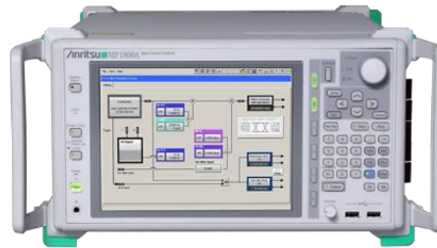
Bit error rate tester, BERT
